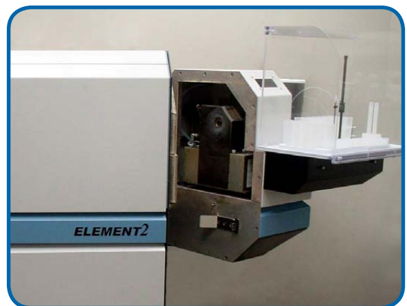
SC-E2 Moves with ELEMENT 2 door to easily replace cones without removing the autosampler.
