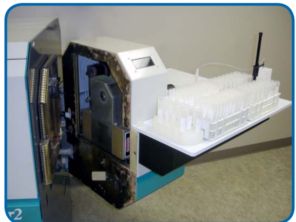
SC-E4 Moves with ELEMENT 2 door to easily replace cones without removing the autosampler.
