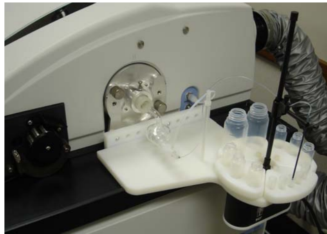
SC Prime with shelf to integrate directly to the PerkinElmer ELAN DRC ICPMS
